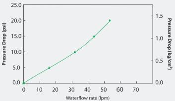
0.2µm AseptiSure® WS, 20" Standard Cartridge Filters
