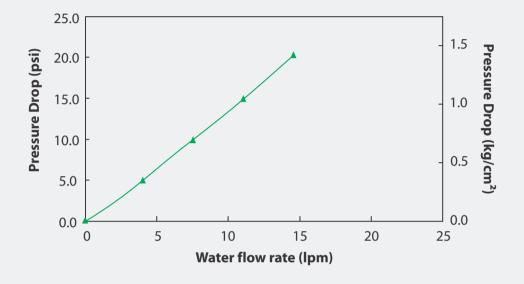
0.2µm AseptiSure® WS, 5" Mini Cartridge Filters
